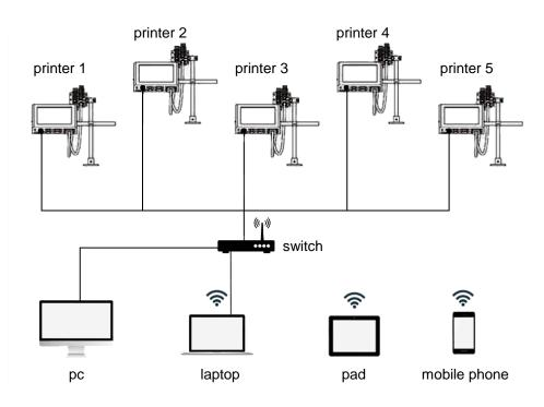
One user terminal controls multiple printing devices, which realizes multiple printers working in time sequence, and makes the production line intelligent. This also provides remote troubleshooting of the printer thus giving maximum uptime.
