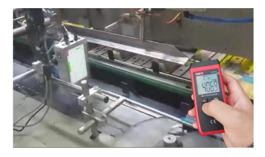
The printing trigger action can be controlled within 10 milliseconds. The maximum printing speed can reach 406 meters / minute, which is about 150% of similar products.
