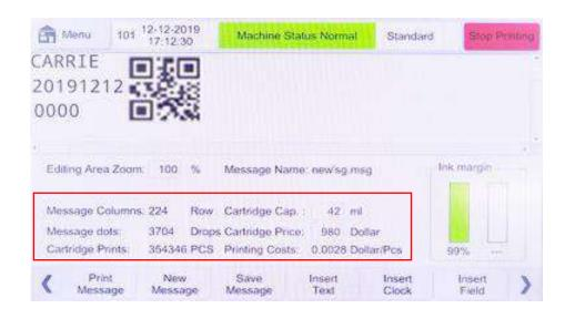
The system is embedded with a powerful ink drop consumption algorithm, which realizing real-time control of inkjet printing costs, saving 15% of consumables compared with similar products.
