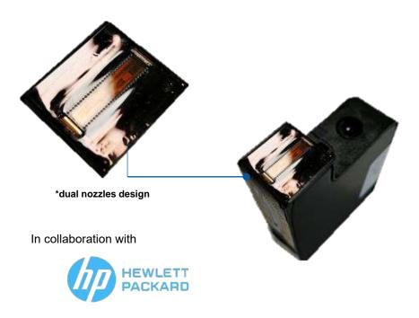
TruCode researched along with Hewlett Packard the "Alternate Printing" model in the industry. The left and right rows of the ink cartridge nozzles work alternately, which avoids the problem of nozzle clogging and also extends the service life of the nozzles.
